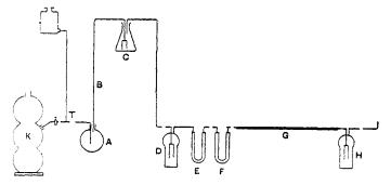
1. The  $5\infty$  cc. distilling flask A in which the phosphine is generated.
